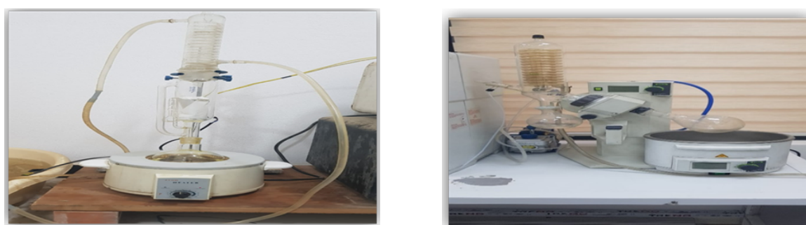
Fig. 2 Soxhlet Extraction of Banana Peels and Concentration of the Extract Using a Rotary Evaporator
