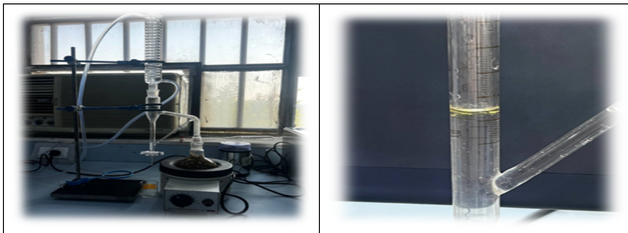
Fig. 2 Clevenger apparatus to extract essential oil of Artemisia vulgaris
